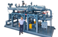
Fuel oil pump and heater set rated for 10,000 gph with steam HEX and 200 KW electric heater
