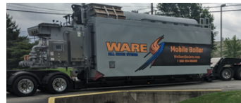
Trailer Mounted Rental Boilers
